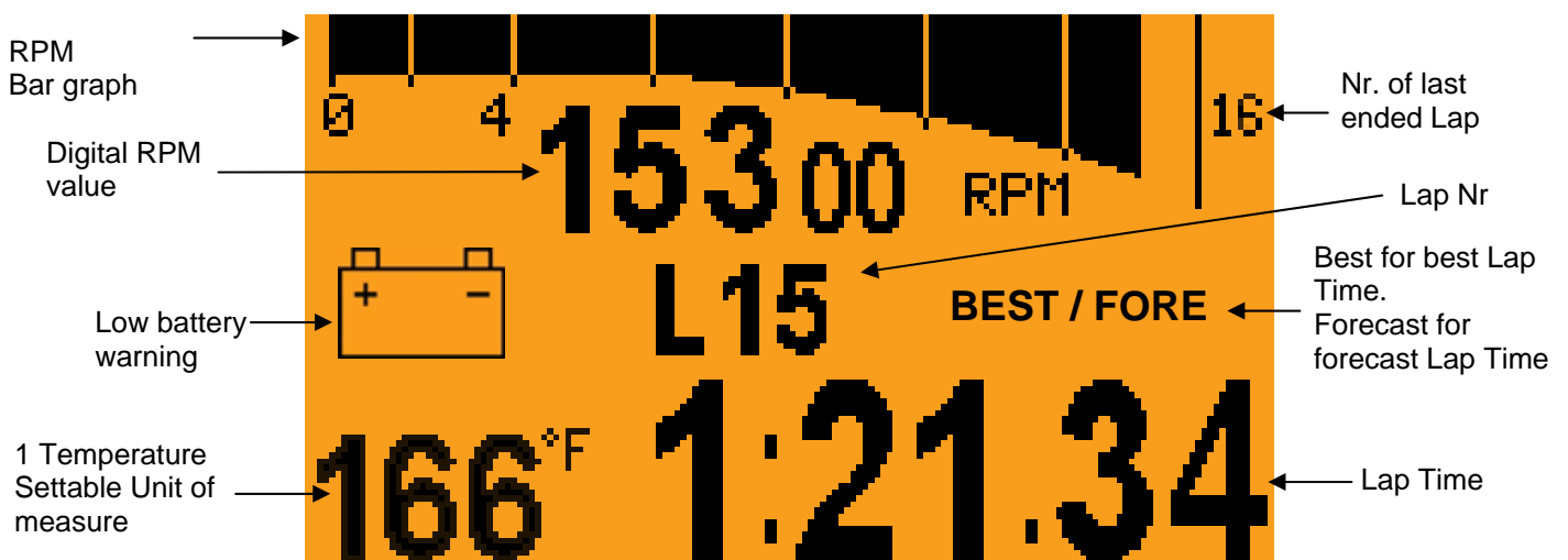
Figure 2: Display Description MyChron 4 on line.
