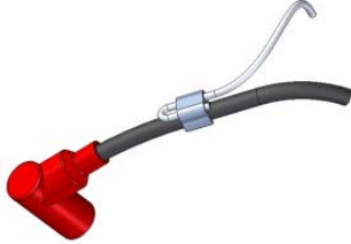
Wrapping of RPM cable on spark cable
