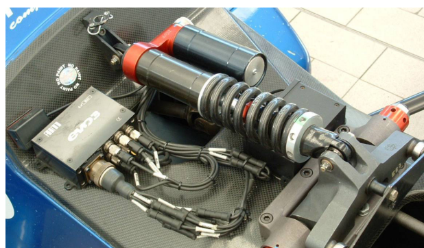
Figure 3: EVO 3 installation on a FR2000
