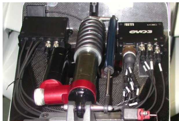
Figure 2: EVO 3 installation on a FR2000
